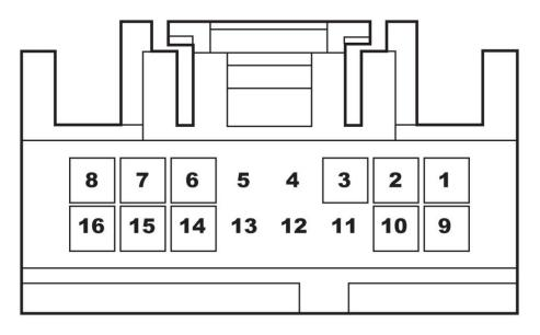
This is the pin view of the connector in the vehicle
