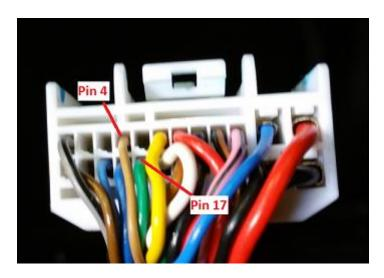
This is the wire view of the radio connector in the vehicle **NOTE**: Wire colors may vary between vehicles but the pin locations are the same.
