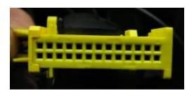
This is the pin view of the radio connector in the vehicle
