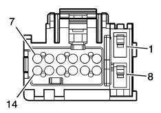
This is the pin view of the connector in the vehicle
