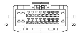
This is the wire view of the connector in the vehicle
